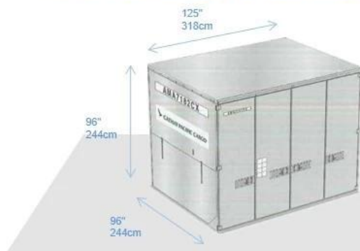
Type: AMA CONTAINER ATA Code: M1 Internal Volume: 621cu. ft 17.58 mc
