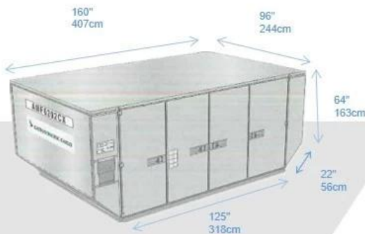
Type: AMF CONTAINER ATA Code: LD36 Internal Volume: 516cu. ft 14.6 mc
